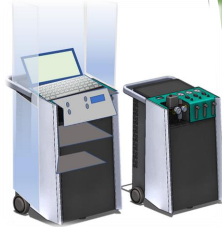
Figure 2: Design of the e-PNose system in conjunction with the gas generator (N 2 )
